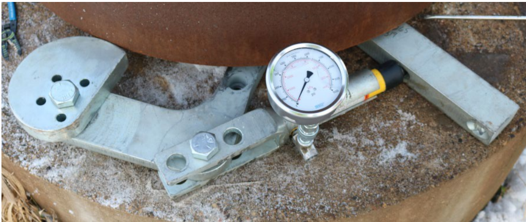
Figure 3.3.24. Millerbernd wrench operation at closest setting
