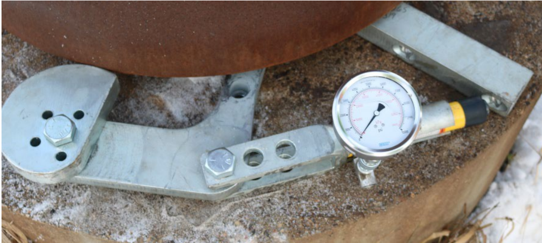
Figure 3.3.25. Millerbernd wrench operation at farthest setting
