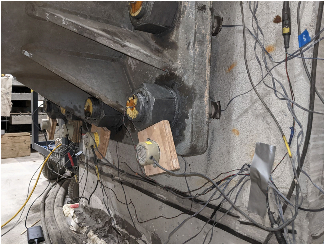
Figure 5.1.3: Lower Post Instrumentation
