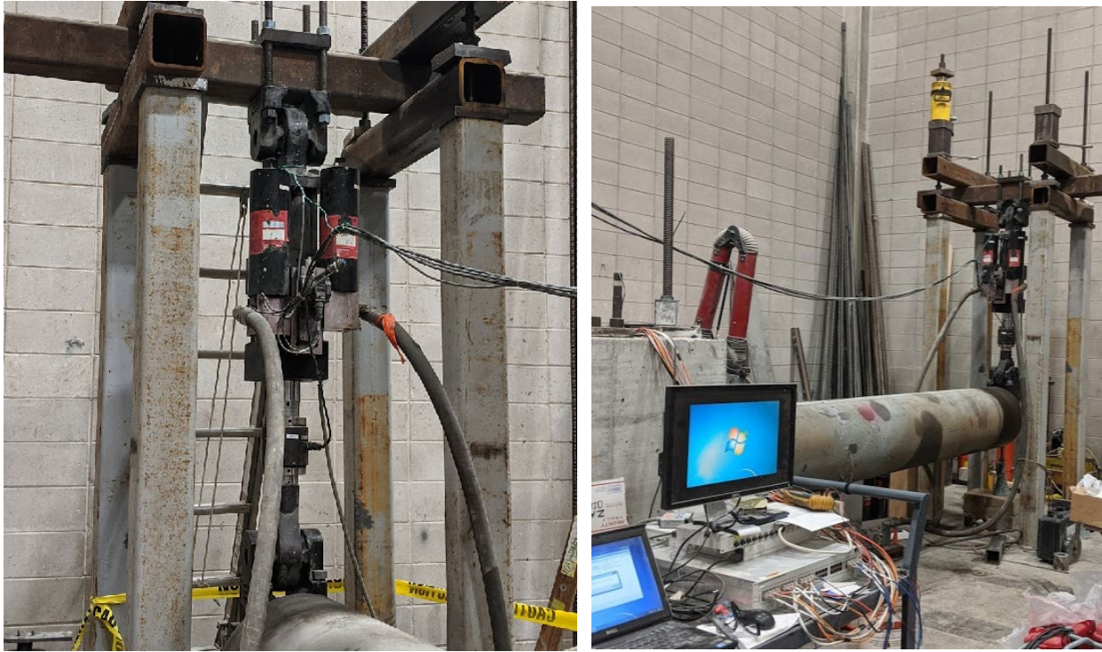
Figure 5.1.5: (Left) MTS Hydraulic Actuator and (Right) Data Acquisition System and Loading Frame
